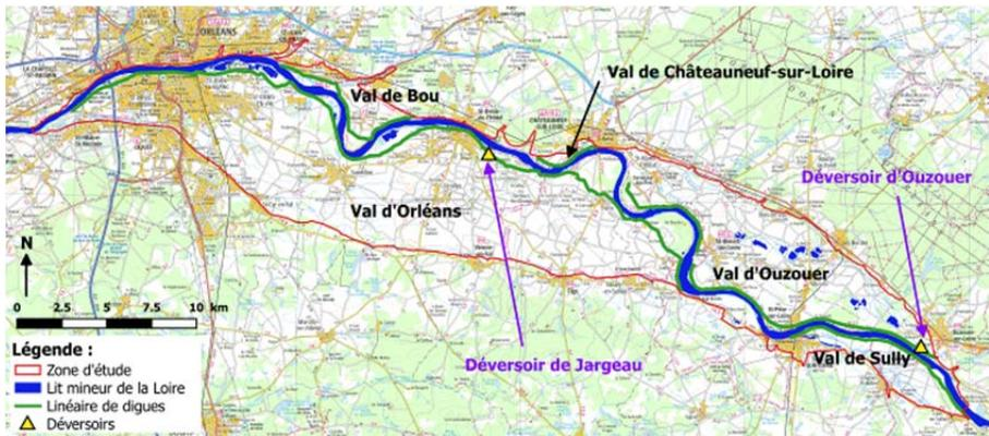
FIGURE 3 - DESCRIPTION DE LA ZONE D'ETUDE ET DES DIFFERENTS SYSTEMES D'ENDIGUEMENT LA COMPOSANT (Source: Scan 100® – IGN©)
